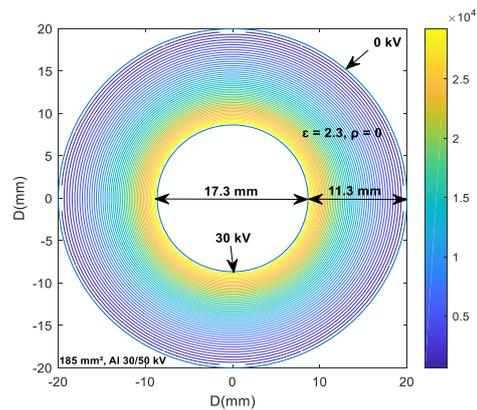
Fig. 2. Potential distribution in XLPE cable with geometry, specification of dielectric and boundary conditions
