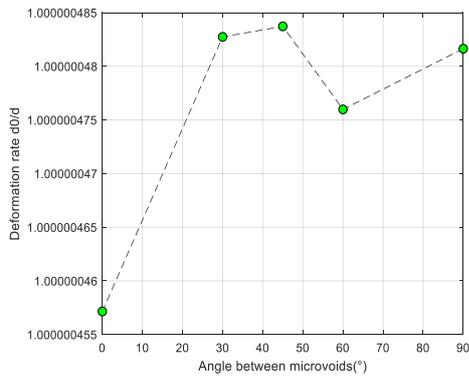
Fig. 4. Deformation rate of microcavity walls versus the angle between defects
