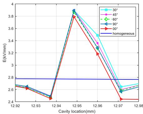
Fig. 3. Electric constraint in the 1<sup>st</sup> defect by different positions of the second microcavity
