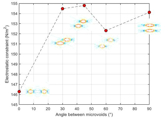
Fig. 5. Electrostatic constraint in the 1<sup>st</sup> defect versus the angle between microcavities
