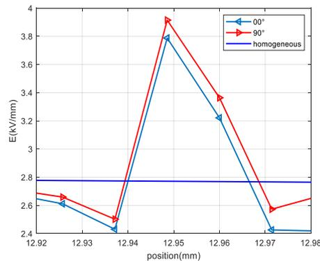
Fig. 6. Electric constraint in the 1<sup>st</sup> defect: the case of three cavities by different positions
