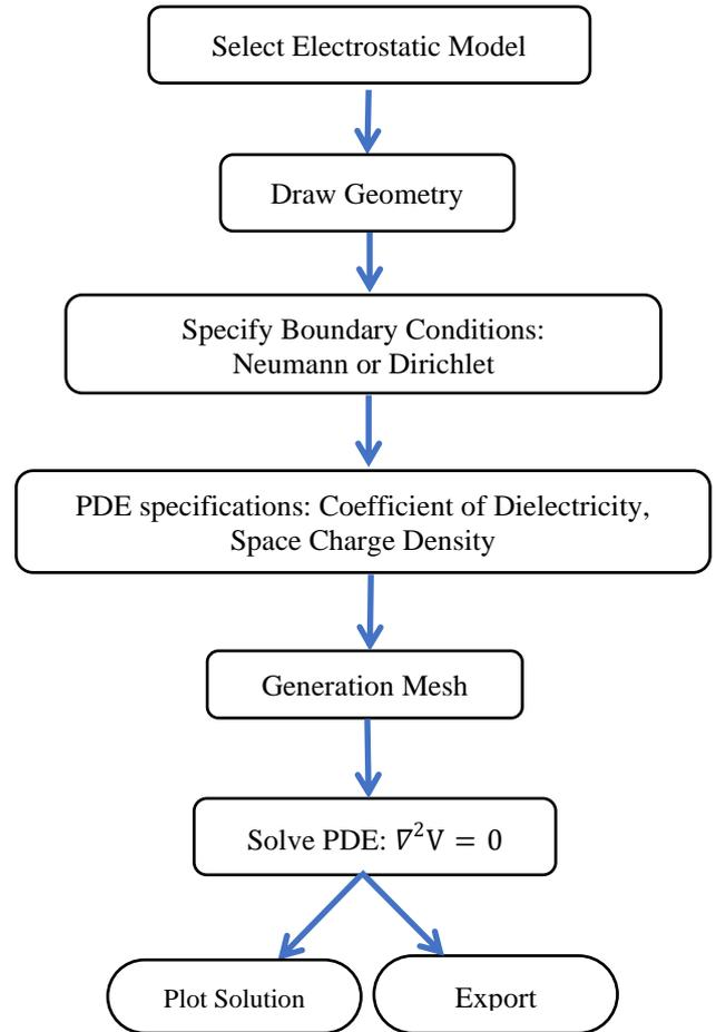
Fig. 1. Flowchart of the steps to put the FEM model of the cable on the PDE Toolbox of MATLAB
